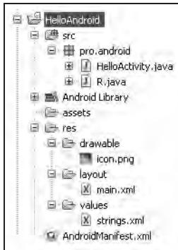
Figure 2-7. The structure of the “Hello World!” app
